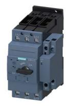
Circuit breaker size S2 for motor protection, CLASS 10 with overload relay function A-release 18...25 A N-release 325 A Screw terminal Standard switching capacity
