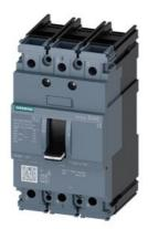
circuit breaker 3VA5 UL frame 125 breaking capacity class S 25kA @ 480 V 3-pole, line protection TM210, FTFM, In=110A overload protection Ir=110A fixed short-circuit protection li=10 x In UL489 SB (naval), 50 deg. cel. nut keeper kit on both sides
