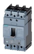
circuit breaker 3VA5 UL frame 125 breaking capacity class M 35kA @ 480 V 3-pole, line protection TM240, ATAM, In=20A overload protection Ir=16A ...20A short-circuit protection Ii=7.5...15 x In cable connection on both sides
