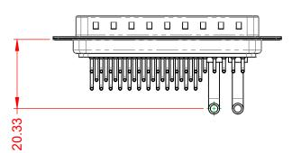
POWER/CO-AX CONTACT RATING:30A (CURRENT)(IF PRESENT)SIGNAL CONTACT CURRENT RATING:5A PER CONTACTSIGNAL CONTACT RESISTANCE:10mΩ MAX.INSULATOR RESISTANCE:5000MΩ min.DIELECTRIC5000MΩ min.
