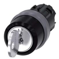
RONIS key-operated switch, 22 mm, round, plastic with metal front ring, lock number SB30, with 2 keys, 3 switch positions I>O<II, momentary contact type, actuating angle 2x45°, 10:30h/12h/13:30h, key removal O, possible special locks: SB31, 421, 455 Z=50-unit packaging
