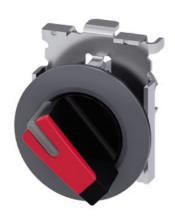
Selector switch, illuminable, 30 mm, round, Metal, matte, red, selector switch, short, front ring for flush installation, 2 switch positions O-I, latching, actuating angle  $90^{\circ}$ , 10:30h/13:30h, with laser labeling, upper case
