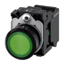
Illuminated pushbutton, 22 mm, round, plastic, green, pushbutton, flat, momentary contact type, with holder, 1NO, LED module with integrated LED 24 V AC/DC, spring-type terminal, with laser labeling, upper case and lower case, always upper case at beginning of line
