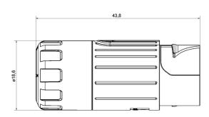
Main Dimensions Extension \*for max. wire cross-section pay attention to the cross-section of used contacts
