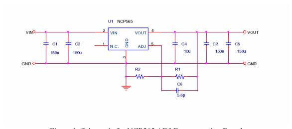
Figure 1: Schematic for NCP565 ADJ Demonstration Board
