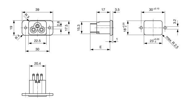
E: Solder terminals short: 18.9 mm E: Solder terminals long: 22.6 mm
