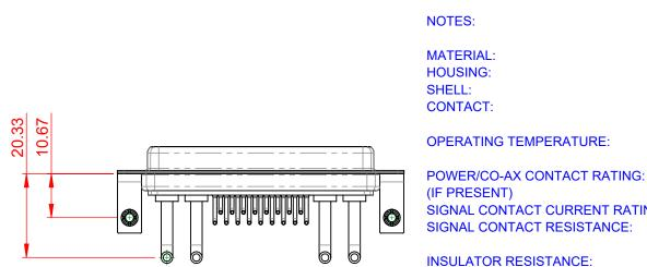
THERMOPLASTIC POLYESTER, UL94V-0 STEEL, NICKEL PLATED COPPER ALLOY, 30µ GOLD PLATED
