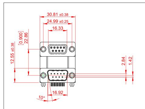
THIS IS A C.A.D. GENERATED DRAWING TOLERANCE UNLESS OTHERWISE SPECIFIED DO NOT MAKE MANUAL REVISIONS TO MASTER. .X ±0.25 .XX ±0.13 .XXX ±0.10 6 5.8 U 6.0 3.18 ±0.38 19.6
