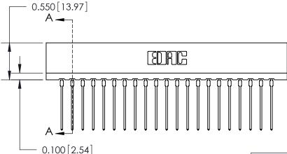
Note: MBB switching contacts assembled in specified positions are available on request. 717 Series Ultra-Mate Card Edge Connector - Press Fit Part Number: 717-042-541-201
