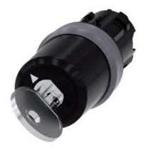
key-operated switch Siemens, 22 mm, round, plastic with metal front ring, lock number SSG10, with 2 keys, 2 switch positions O-I, latching, actuating angle 90°, 10:30h/13:30h, key removal I, Z=50-unit packaging
