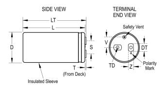
Series ALS70 Dielectric Aluminum Electrolytic Description Screw Terminal, Aluminum Electrolytic RoHS AEC-Q200 No Halogen Free Yes Component 300 g Weight Dimensions D And L Include Sleeving. MS (MxH) = Notes M12x16. Mounting Clamp (Sold Separately): V4/2737 Shelf Life 156 Weeks
