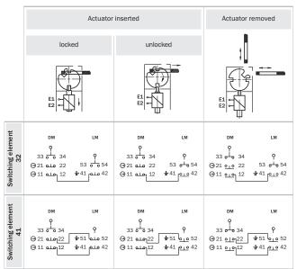
$<sup>\</sup>frac{1}{\mathbf{P}}$  Positive action N/C locking monitoring contact
