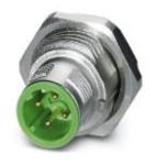
Bus system flush-type plug, with green contact carrier, 4-pos., M12 SPEEDCON, shielded, D-coded, rear/ screw mounting with M16 thread, with straight solder connection
