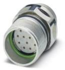
Device connector for front wall, straight, shielded: yes, for standard and SPEEDCON interlock, M23, No. of pos.: 16+3, type of contact: Socket, Solder connection, Axial seal, Central fastening M20 x 1.5, can be positioned via a locking nut
