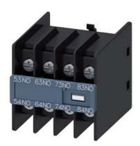
Auxiliary switch on the front, 4 NO Current path 1 NO, 1 NO, 1 NO, 1 NO for contactor relays Size S00 Ring cable lug connection 53/54, 63/64, 73/74, 83/84 Physically coded; only with contactor relays 3RH2140\* and 3RH2440\* can be combined (according to EN 50011)
