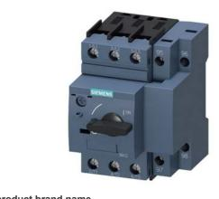
Circuit breaker size S0 for motor protection, CLASS 10 with overload relay function A-release 18...25 A N-release 325 A Screw terminal Standard switching capacity
