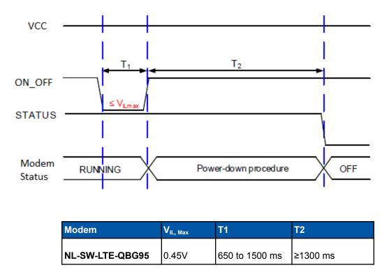
Due to architecture changes to the chipset, the nRESET signal and the ON\_OFF signal are internally tied together inside of the Quectel module used on the modem. This pin should not be permanently attached to ground, nor should this pin be driven high or have a pull up resistor applied. The ON\_OFF signal should be driven with an open collector output or with an open collector transistor. The signal is internally pulled up to 1.5V and should not be driven high, doing so may damage the modem.
