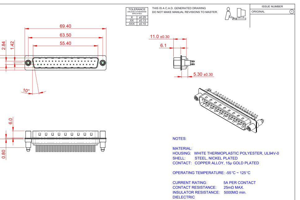
WITHSTANDING VOLTAGE: 1000V AC rms
