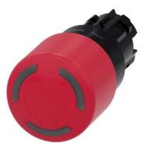
EMERGENCY STOP mushroom pushbutton, illuminable, 22 mm, round, plastic, red, 30 mm, positive latching, acc. to EN ISO 13850, rotate-tounlatch, with laser labeling, inscription or symbol Customer-specific selection with SIRIUS ACT configurator (CIN)
