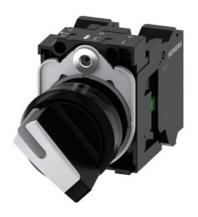
Selector switch, illuminable, 22 mm, round, plastic, white, selector switch, short, 2 switch positions O-I, latching, 10:30h/13:30h, with holder, 1 NO, 1 NC, spring-type terminal, with laser labeling, upper case and lower case, always upper case at beginning of line
