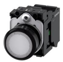
Illuminated pushbutton, 22 mm, round, plastic, white, pushbutton, flat, momentary contact type, with holder, 1NO, LED module with integrated LED 110 V AC, spring-type terminal, with laser labeling, symbol number according to, ISO 7000 or IEC 60417
