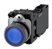
Illuminated pushbutton, 22 mm, round, plastic with metal front ring, blue, pushbutton, flat, momentary contact type, with holder, 1 NO+1 NC, LED module with integrated LED 24 V AC/DC, screw terminal, with laser labeling, upper case
