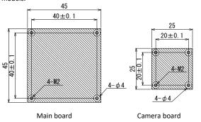
Do not install metallic parts for mounting on the shaded areas.
