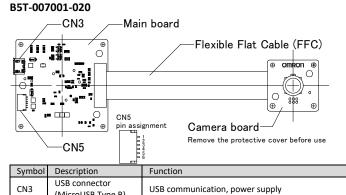
CN5 UART connector UART communicationl, power supply, reset input Limit the coupling of CN3 and CN5 to less than 10 times.
