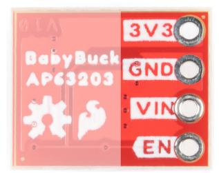
Both the Buck Regulator as well as the Baby Buck Regulator ratchet the output voltage down to **3.3V**. Be mindful that thermal properties change as Vin increases.
