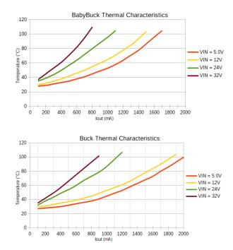
To dissipate some of the excess heat, we've added a copper pad for a heat sink on the back of the 1" x 1" Buck Regulator Board. Use one of our small heatsinks and attach it with some thermal tape.
