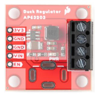
The Baby Buck sacrifices flexibility for space. Use the plated through holes for input and output power.
