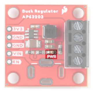
To disable this LED, cut the Jumper on the back of the board:
