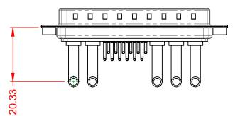
POWER/CO-AX CONTACT RATING:40A (CURRENT)(IF PRESENT)SIGNAL CONTACT CURRENT RATING:5A PER CONTACTSIGNAL CONTACT RESISTANCE: $10m\Omega$  MAX.INSULATOR RESISTANCE:5000MΩ min.DIELECTRICDIELECTRIC
