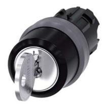
RONIS key-operated switch, 22 mm, round, plastic with metal front ring, lock number SB30, with 2 keys, 3 switch positions I>O<II, momentary contact on the left, latching on the right, actuating angle 2x45°, 10:30h/12h/13:30h, Key removal O+II, possible special locks: SB31, 421, 455, with laser labeling, upper case and lower case, always upper case at beginning of line
