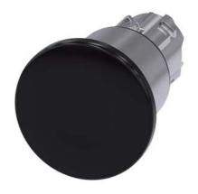
Mushroom pushbutton, 22 mm, round, metal, shiny, black, 40 mm, 3 switch positions, latches after pushing in, unlatches by pull-to-unlatch mechanism to center position, after pulling out the button Retraction to center position, with laser labeling, upper case
