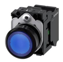
Illuminated pushbutton, 22 mm, round, plastic, blue, pushbutton, flat, momentary contact type, with holder, 1NO, LED module with integrated LED 24 V AC/DC, spring-type terminal, with laser labeling, lower case
