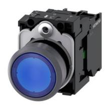
Illuminated pushbutton, 22 mm, round, plastic with metal front ring, blue, pushbutton, flat, momentary contact type, with holder, 1NO, LED module with integrated LED 24 V AC/DC, screw terminal, with laser labeling, inscription or symbol Customer-specific selection with SIRIUS ACT configurator (CIN)
