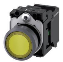
Illuminated pushbutton, 22 mm, round, plastic with metal front ring, yellow, pushbutton, flat, momentary contact type, with holder, 1NO, LED module with integrated LED 24 V AC/DC, spring-type terminal, with laser labeling, upper case and lower case, Always upper case at the beginning of the word
