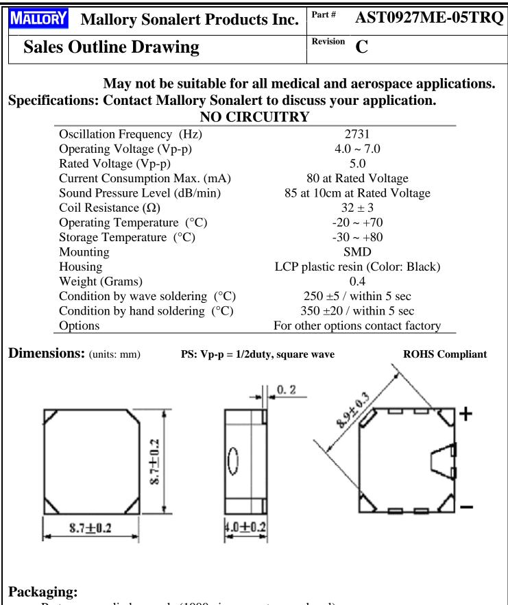
Parts are supplied on reels (1000 pieces per tape and reel). Units do not come with wash label and are not appropriate for aqueous wash.
