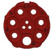
Contact Arrangement mating view
