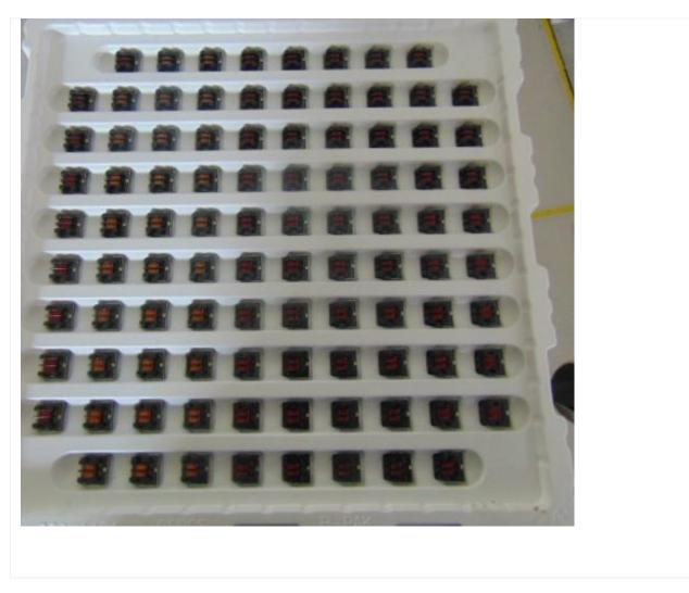
**Impact on Form, Fit, Function, Quality or Reliability**: The upgrade to high temperature wire insulation will have no effect on Form, Fit or Function. To prevent the core crack and offer better protection and improve package quality. TQ/BQ will be change to TQ: 96 PCS/TRAY BQ: 672PCS/BOX from TQ: 29PCS / TUBE and BQ: 725PCS/ BOX.
