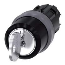
RONIS key-operated switch, 22 mm, round, plastic with metal front ring, lock number SB30, with 2 keys, 3 switch positions I>O<II, momentary contact on the left, latching on the right, actuating angle 2x45°, 10:30h/12h/13:30h, Key removal O+II, possible special locks: SB31, 421, 455, with laser labeling, lower case
