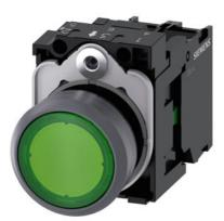
Illuminated pushbutton, 22 mm, round, plastic with metal front ring, green, pushbutton, flat, momentary contact type, with holder, 1NO, LED module with integrated LED 110 V AC, screw terminal, with laser labeling, symbol number according to, ISO 7000 or IEC 60417
