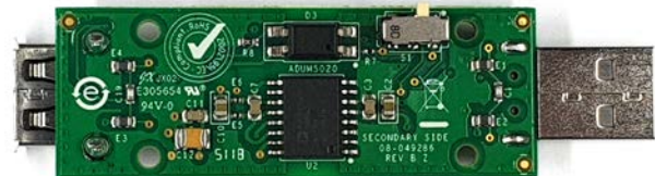
Figure 3. S1 Switch Position for Full Speed Operation
