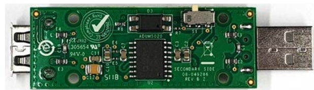
Figure 4. S1 Switch Position for Low Speed Operation
