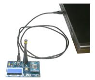
Connect the Programming Docks to a computer with the cables included with the kit. USB drivers are on the website so install them if prompted by the computer.
