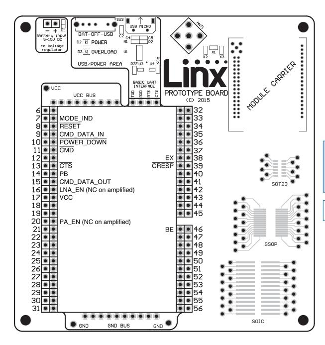
Warning: Installing or removing a Carrier Board while power is applied could cause permanent damage to the module. Either turn off power to the board or unplug the USB cable before installing or removing a Carrier Board
