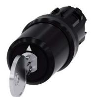
Key-operated switch BKS, 22 mm, round, plastic, lock number S1, with 2 keys, 3 switch positions I>O<II, momentary contact type, actuating angle 2x45°, 10:30h/12h/13:30h, key removal O, with laser labeling, inscription or symbol Customer-specific selection with SIRIUS ACT configurator (CIN)
