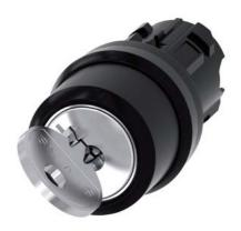
RONIS key-operated switch, 22 mm, round, plastic, lock number SB30, with 2 keys, 2 switch positions O-I, latching, actuating angle 90°, 10:30h/13:30h, key removal I, possible special locks: SB31, 421, 455, with laser labeling, lower case
