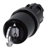
Key-operated switch IKON, 22 mm, round, plastic, lock number 360012K1, with 2 keys, 3 switch positions I-O-II, latching, actuating angle 2x45°, 10:30h/12h/13:30h, Key removal I+O+II Z=50-unit packaging
