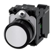
Pushbutton, 22 mm, round, plastic, white, pushbutton, flat, momentary contact type, with holder 1 NO, spring-type terminal, with laser labeling, upper case and lower case, always upper case at the beginning of the word
