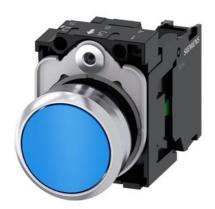
Pushbutton, 22 mm, round, metal, shiny, blue, pushbutton, flat, momentary contact type, 1 NO, screw terminal, with laser labeling, inscription or symbol Customer-specific selection with SIRIUS ACT configurator (CIN)
