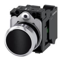
Pushbutton, 22 mm, round, metal, shiny, black, pushbutton, flat, momentary contact type, 1 NO, spring-type terminal, with laser labeling, inscription or symbol Customer-specific selection with SIRIUS ACT configurator (CIN)
