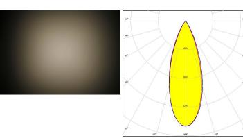
LUMILEDS LED LUXEON MZ FWHM / FWTM 36.0° / 63.0° Efficiency 66 % Peak intensity 1.5 cd/lm LEDs/each optic 1 White Light colour Required components:
