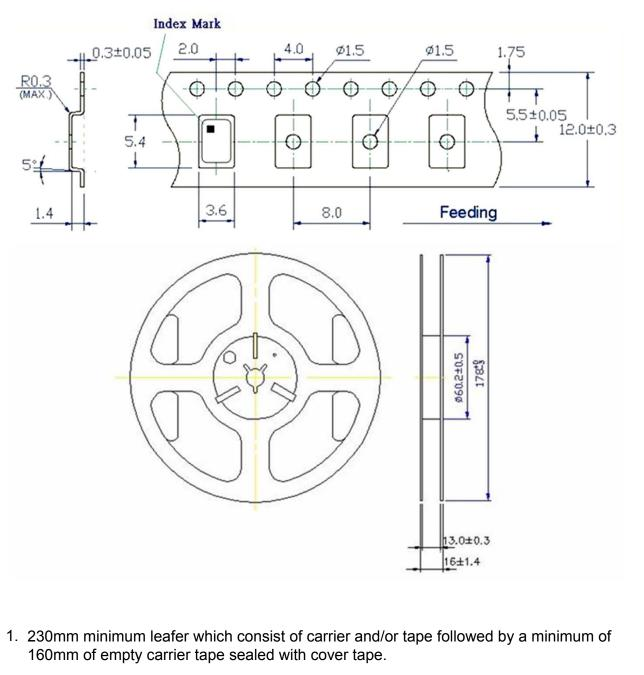
2. 160mm minimum trailer of empty carrier tape sealed with cover tape.
