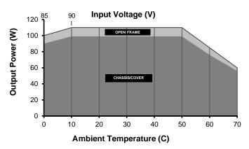
Derating requirements - Derate from 100% load at 50°C to 50% load at 70°C. Derate from 100% load at 90VIN to 90% load at 85VIN. - Derate 10% with Chassis/Cover option.
